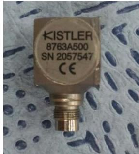
**Figure 4.** KISTLER accelerometer(3 axis)
