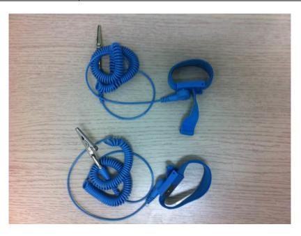
**Description:** Antistatic wrist strap used to safely ground in use of sensitive electronic equipment.
